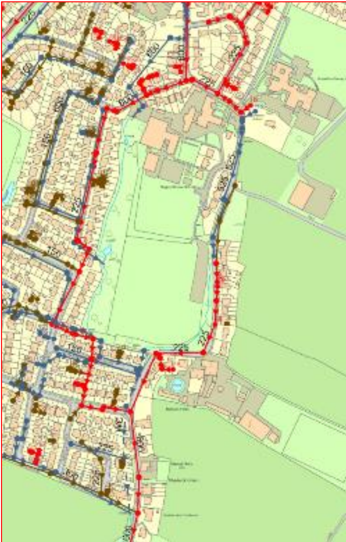
Figure 6: UU Statutory Sewer Map
