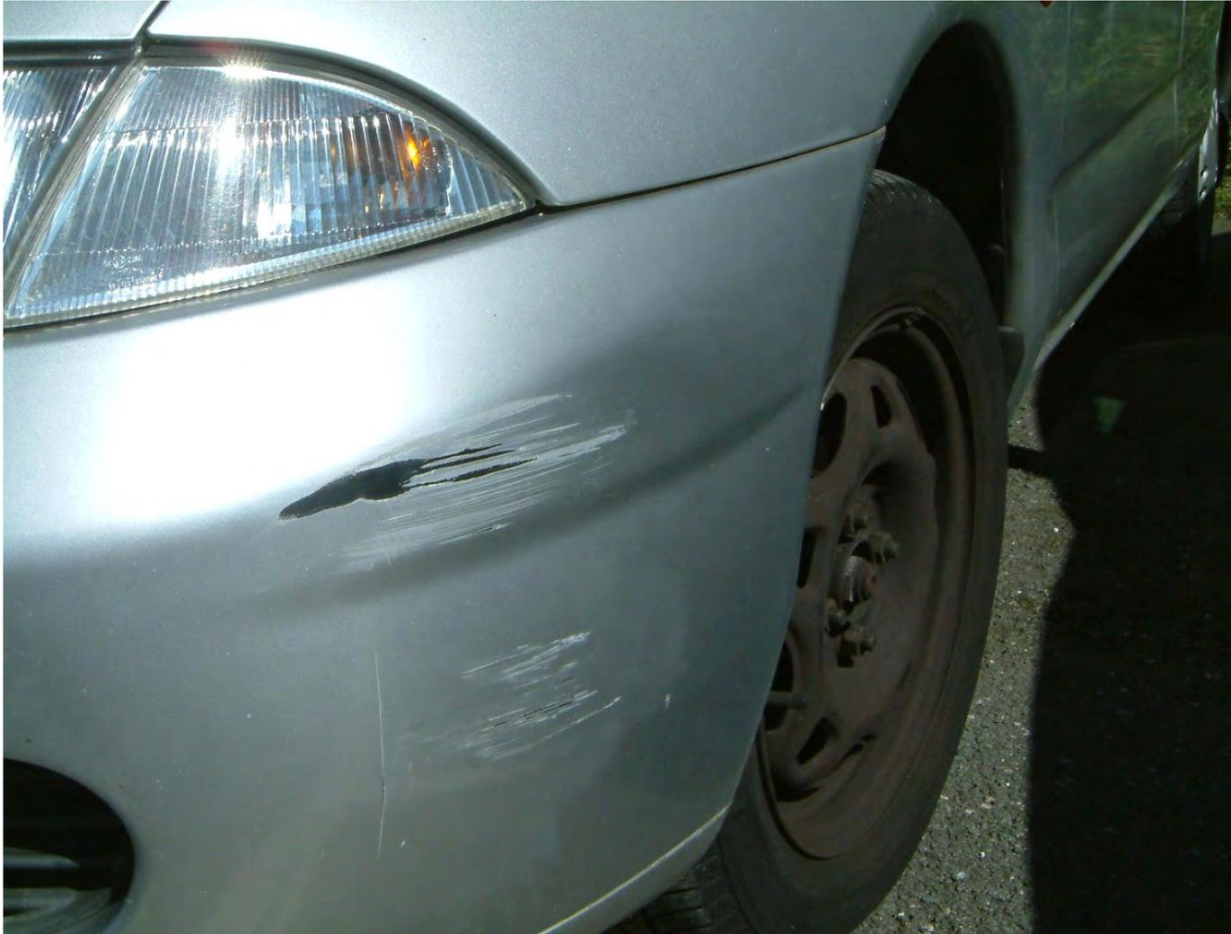
The bumper has excessive abrasions and scratches which detract from the appearance of the vehicle. The vehicle is not in an acceptable condition.
