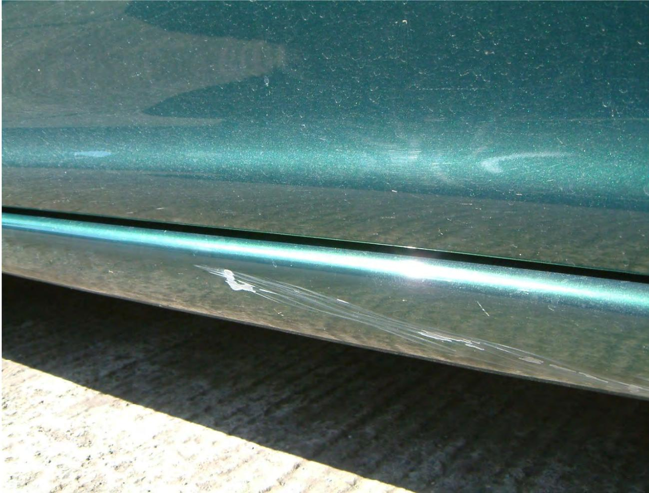
Excessive scratches or abrasions are unacceptable.
