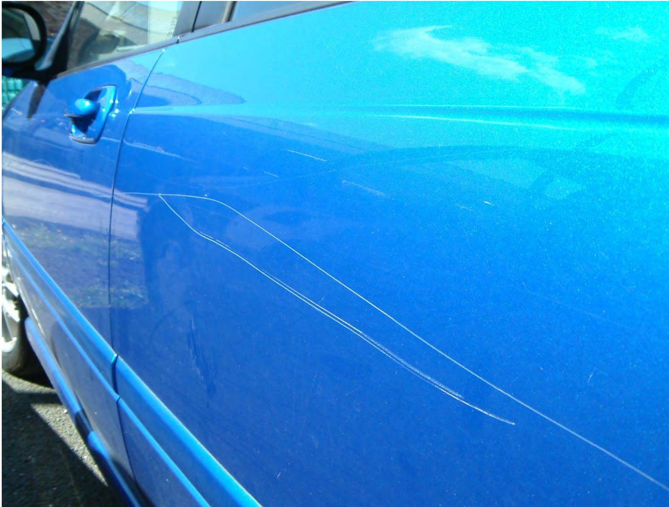
Any scratch of more than 100mm in length is a reason for failure.
