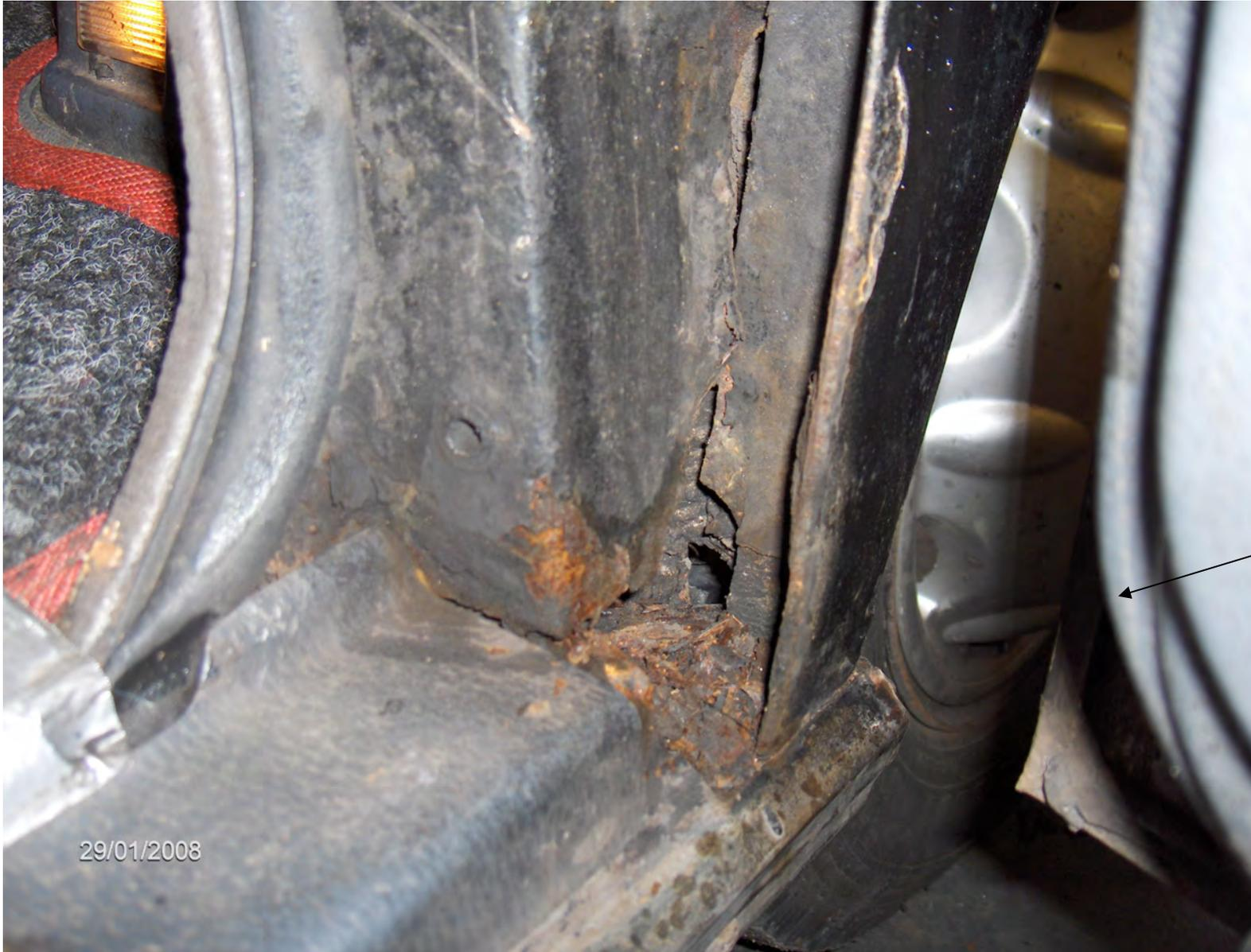
Excessive corrosion at base of C post and sill. A failure item
