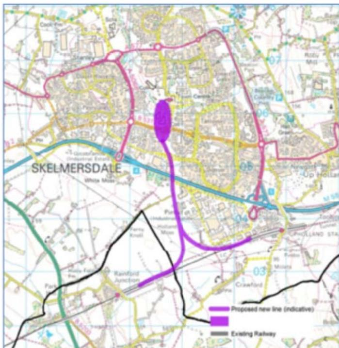
The scheme is shown in Figure 1-A. It involves connections to the railway line between Liverpool and Wigan, running to the south of the town, and a station in the town centre.
