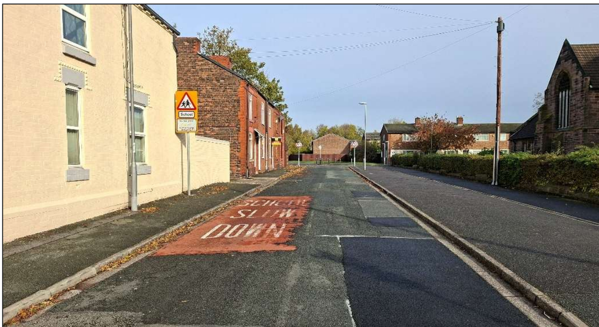
Figure 2.18: Goodban Street - Signage and Road Markings
