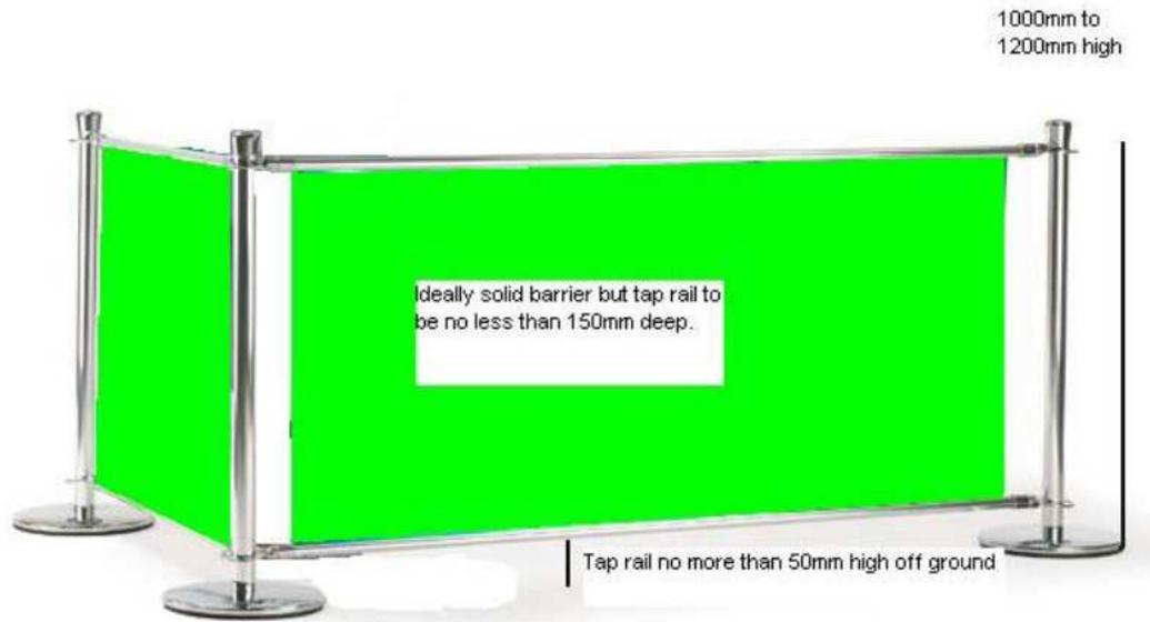
**Image of 1 meter high barrier with top rail 50mm from the ground**
